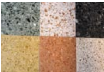
Countertops made with recycled glass and stone chips
